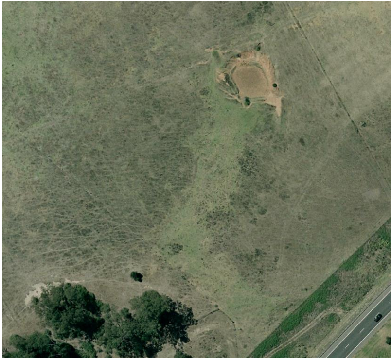
Photo 32 – Drainage line 1, site inspection revealed a grass swale below a small breached Dam 12 (approx. 500m 2 in size)
